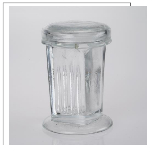
Figure 4.11 Coplin jar used to fix thin smears
